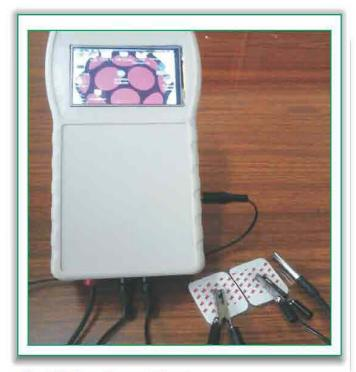
Portable impedance analyzer
